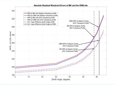
Total (includes implementation errors) WFE On-Axis in the direction of the G.C.
